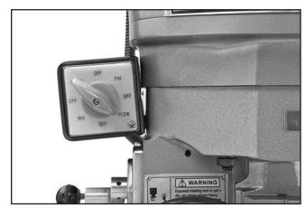
Figure 14. Model G0747 spindle switch.
